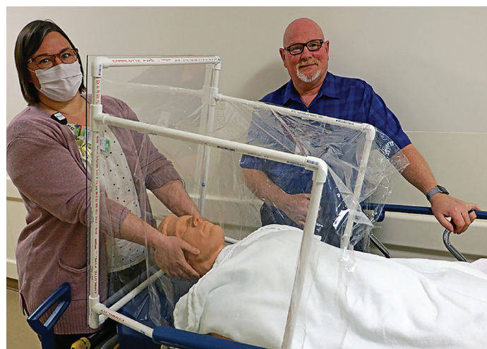
Tomah Health Emergency Services director Suzanne Downing, DNP, RN, left, and hospital Facility Services coordinator Steve Logging test a newly designed portable bed anti-aerosol hood using a mannequin. Downing and Logging developed the unit to protect staff in light of the COVID-19 pandemic.
